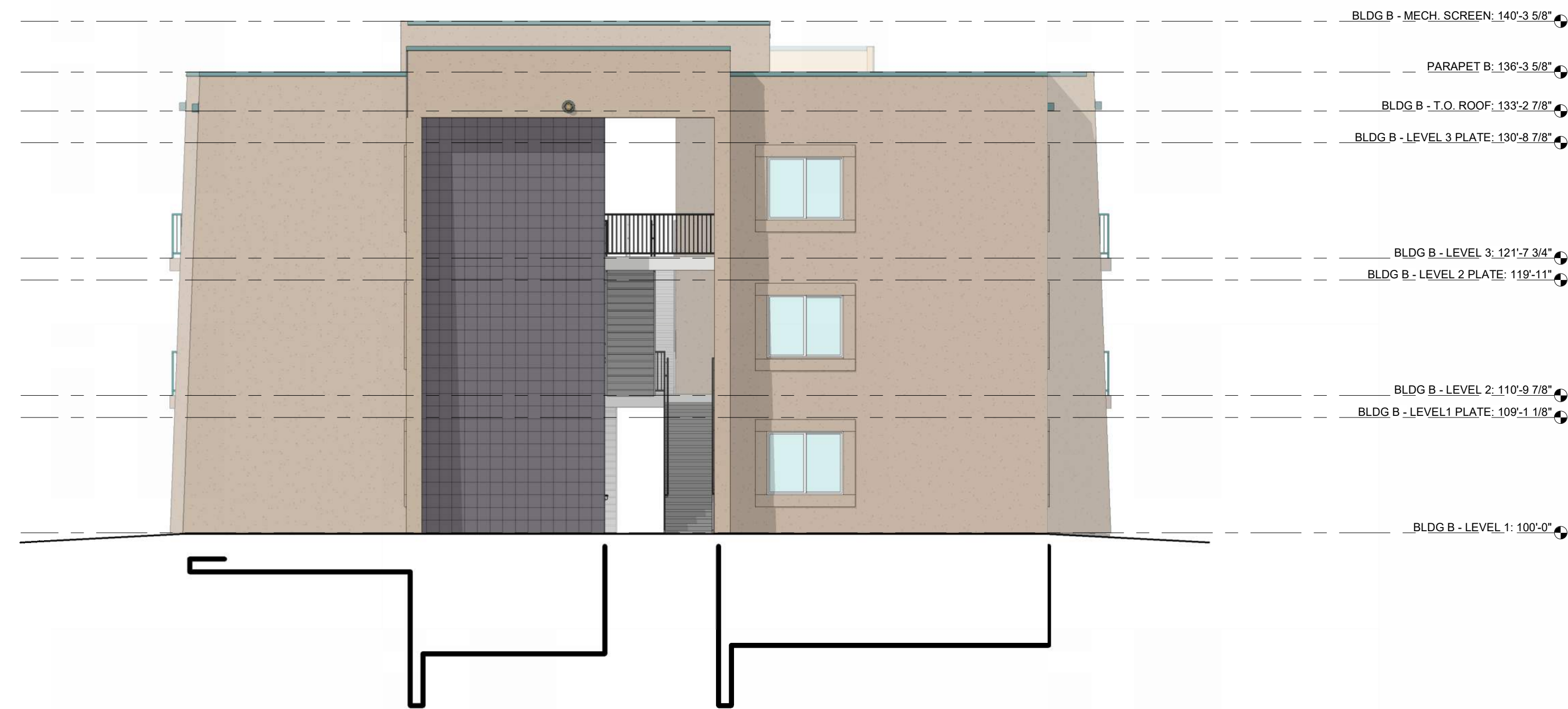
2 RIGHT ELEVATION - BUILDING TYPE B - SD 1/8" = 1'-0"
