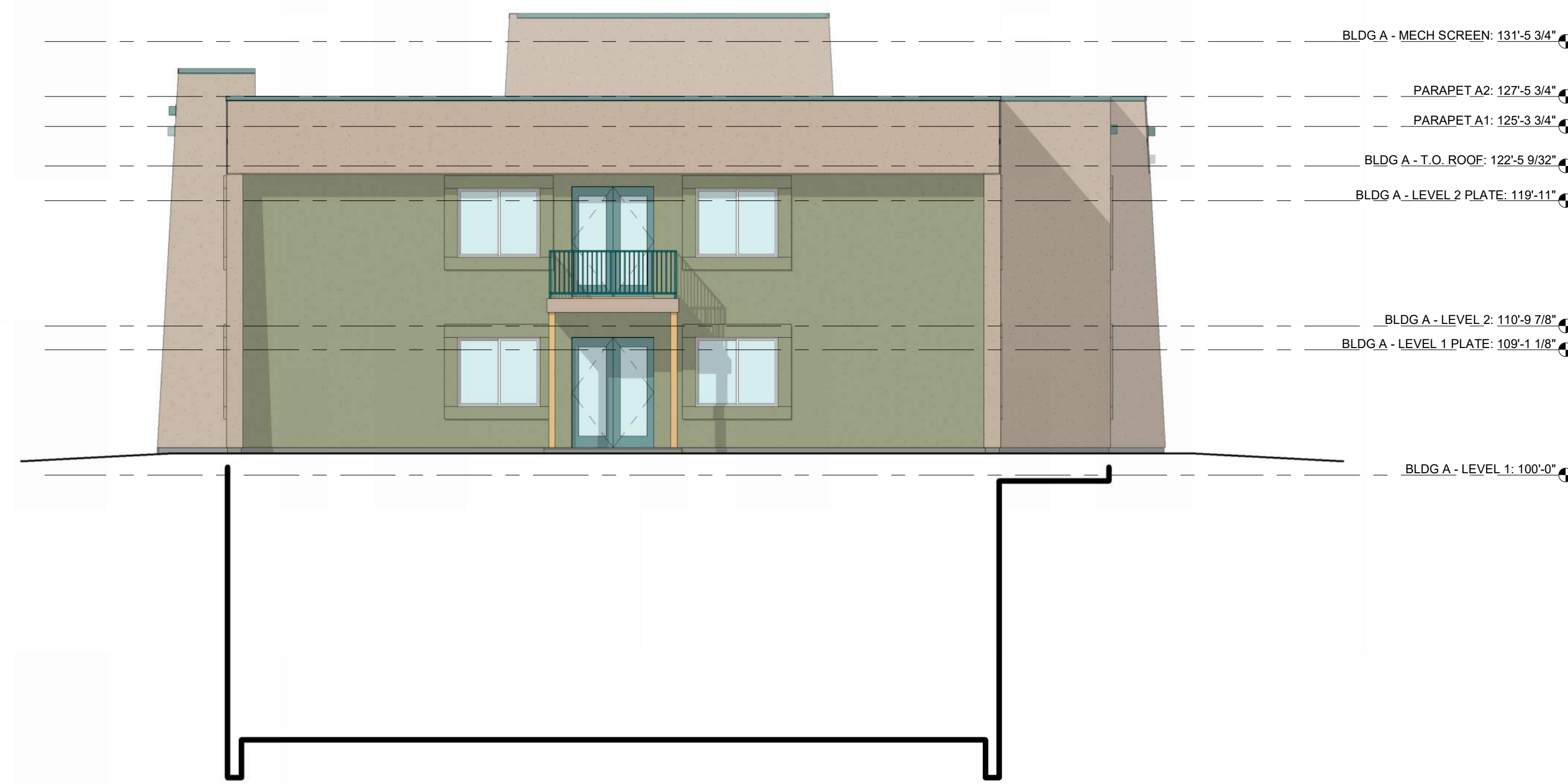
2 RIGHT ELEVATION - BUILDING TYPE A - SD 1/8" = 1'-0"
