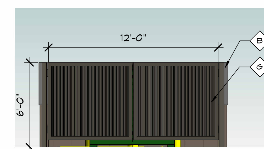
E17 TRASH ENCLOSURE - FRONT 1/4" = 1'-0"
