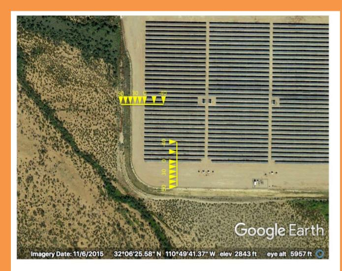
Locations of additional measures of air temperature are marked with yellow triangles. Stations were placed inside the array at 20m and 40m in from the edge of the array, at the edge of the array (0m), and outside the array at 10, 20, 30, 40, and 50m out from the edge of the array to quantify the spatial extent of the PVHI effect.
