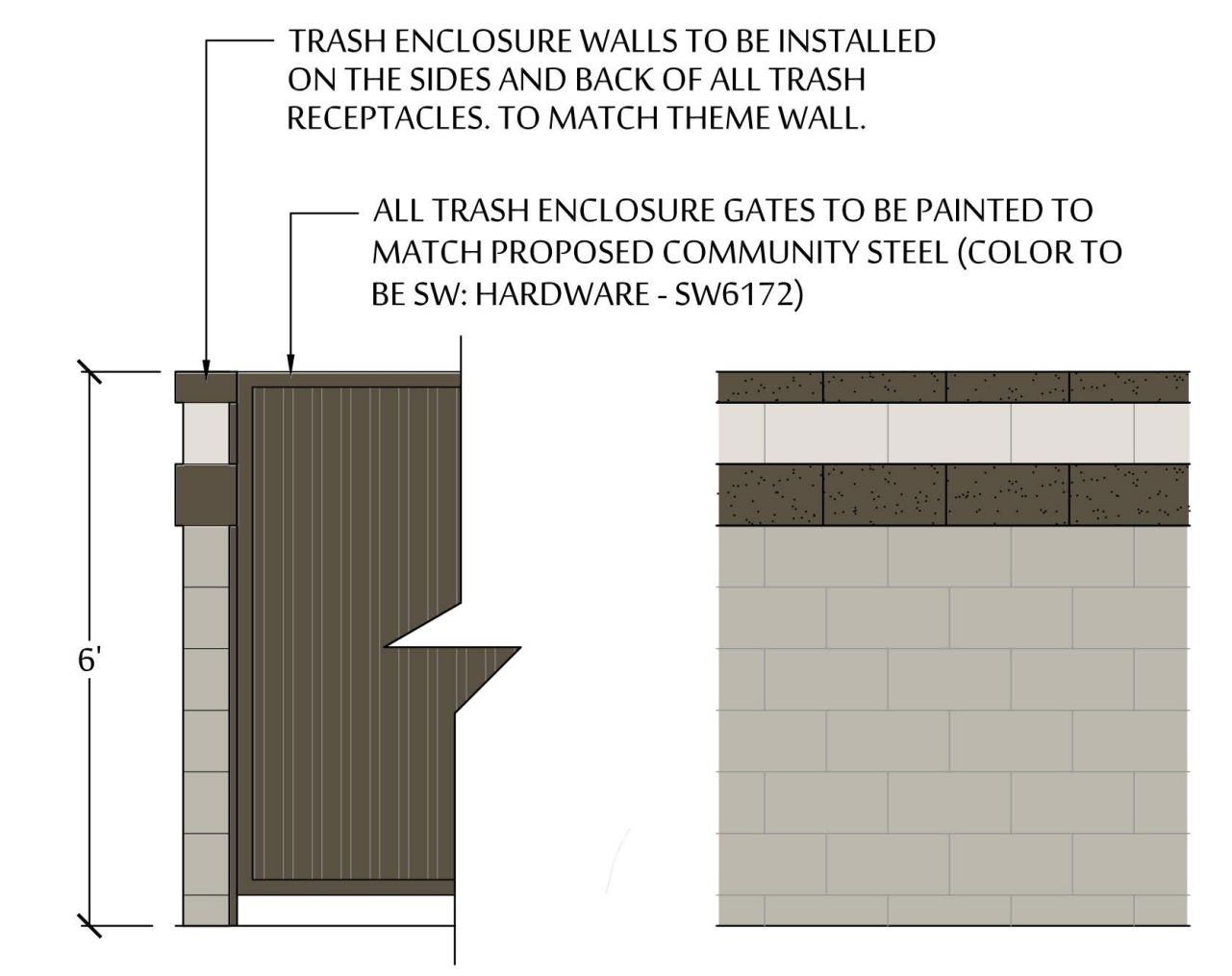
TRASH ENCLOSURE WALL/GATE ELEVATION
