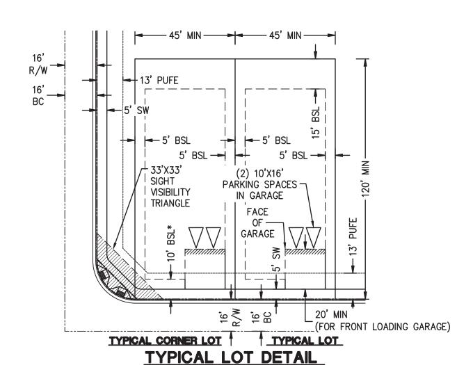
45' x 120' \*MIN 13' BSL FOR LOTS THAT FRONT PUFE PERIMETER SETBACK WHERE SHOWN ON PLAN SCALE: N.T.S.
